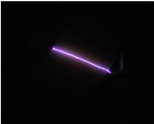
Figure 7. The spark on the surface of the polymer between the electrodes.
