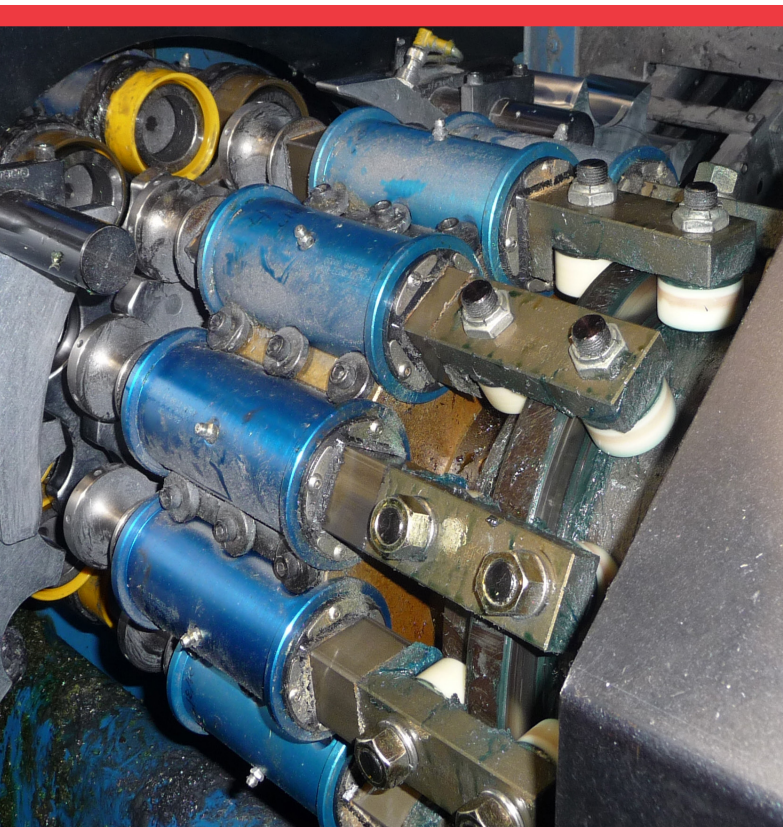
The square ram with polymer cam followers eliminates 720 lubrication points and nearly 1 metric ton of moving mass from the necker.
