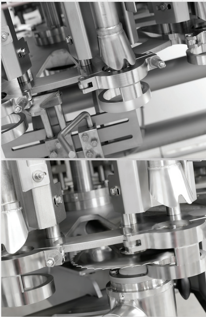
These photos show one of the twelve stations for the FM 8.50 and the cutter blade that separates the bone from the meat.
